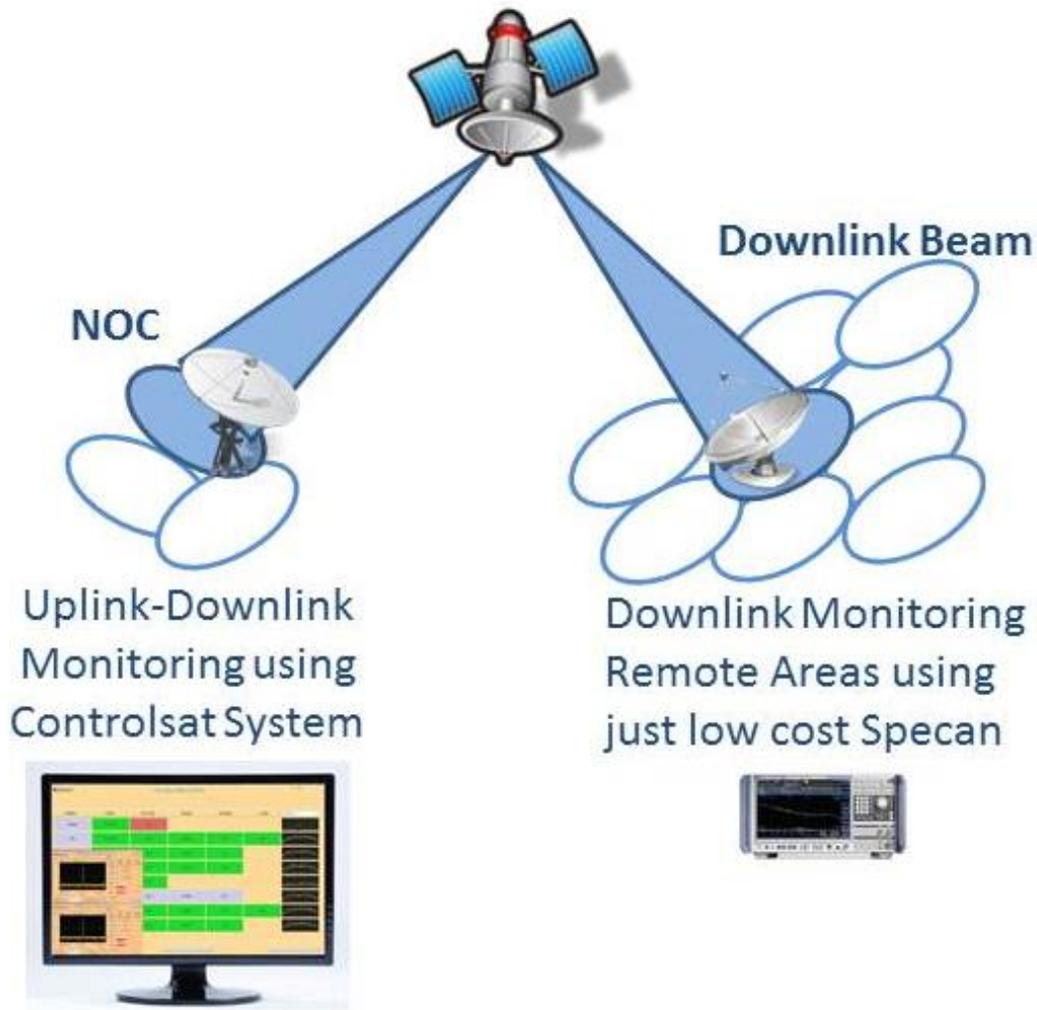
Controlsat installed at the NOC, reads the frequency plan from CMS database and adjusts the thresholds, alarms and warnings automatically and manually depending on the customer requirements. In case there is any interference or a service failure Controlsat automatically detects it and alarm, visually, sound and email reporting.
